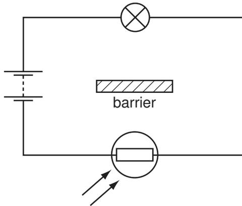
When low intensity light falls on the LDR, the lamp glows dimly.
