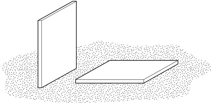
After a few hours, the vertical tile has started to sink into the soft earth, but the horizontal one has not.
